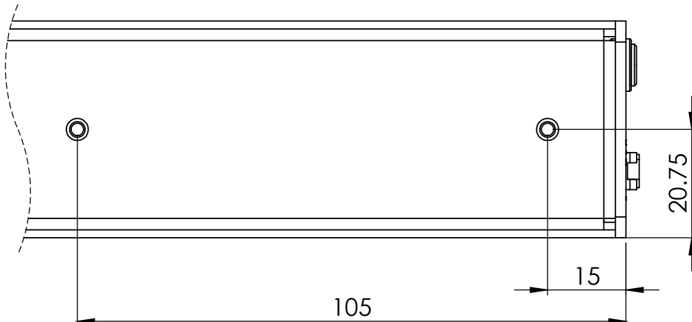
Drawing 8: Mounting points for ACQ1001Q (Single) and ACQ1002R (Rack) Cases
