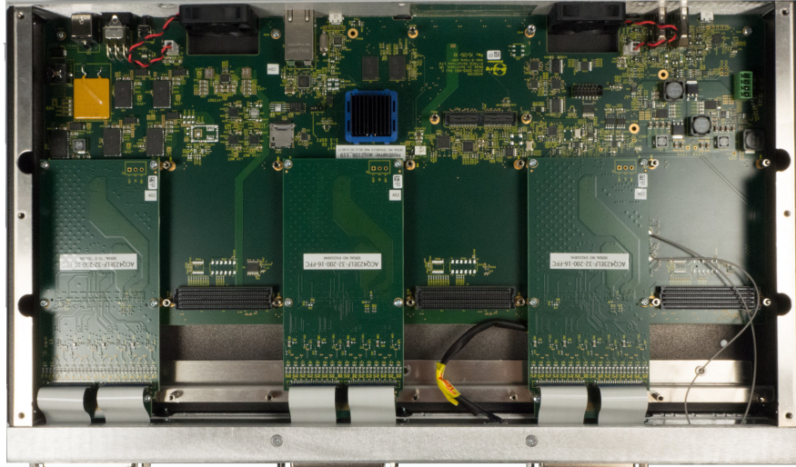
Figure 3: Example Fitted to ACQ2106 Carrier, 96 channels in 1U
