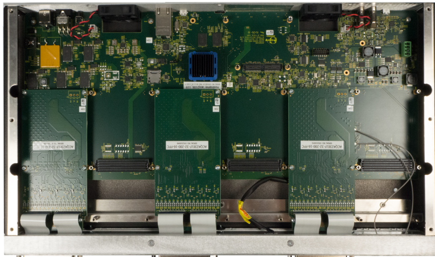
Figure 3: Example Fitted to ACQ2106 Carrier, 96 channels in 1U
