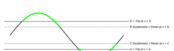
Outside : Thresholds 0xAABBCCDD; B must be > than C
