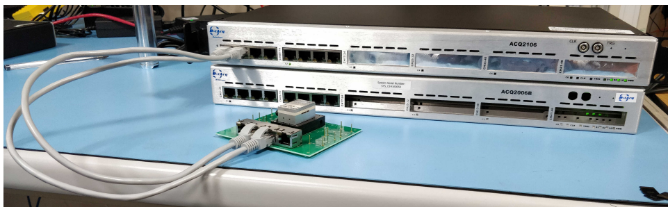
Figure 6: Bolometer connected to a BOLO8 mezzanine in an acq2106 system
