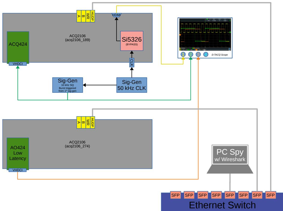
Figure 1: HUDP Demo Hardware Configuration
