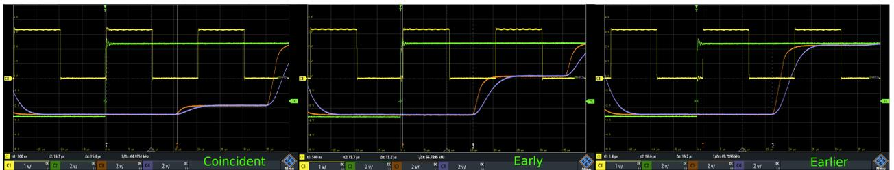
Figure 3: The result of the sample clock sampling the rising edge at various points during the signal slew
