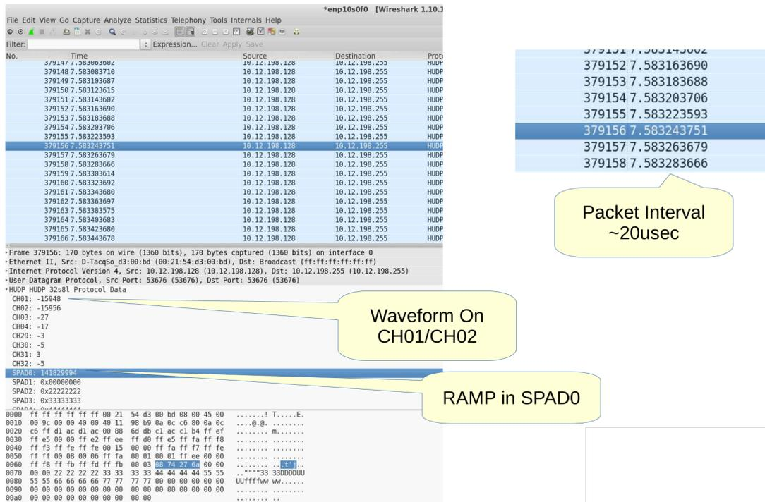
Figure 12: Monitoring packets with Wireshark plugin
