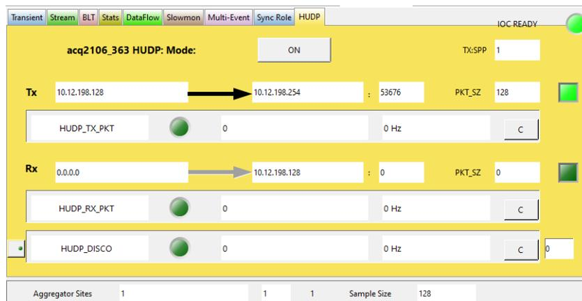
Figure 5: HUDP OPI after configuration by `udp_setup.py`
