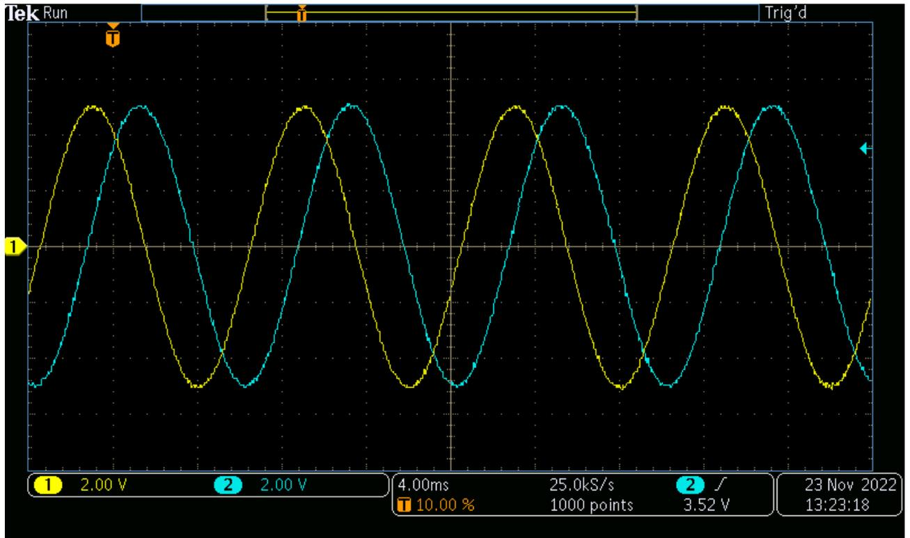
Figure 11: Oscilloscope trace showing data from signal generator in yellow and similar data from DAC in blue
