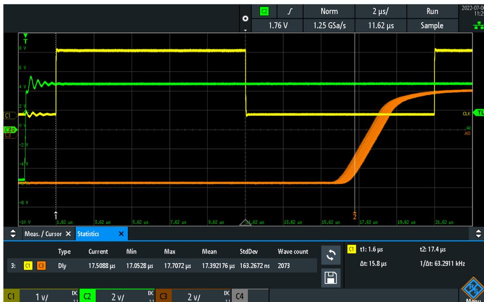
Figure 14: HUDP Latency through Switch
