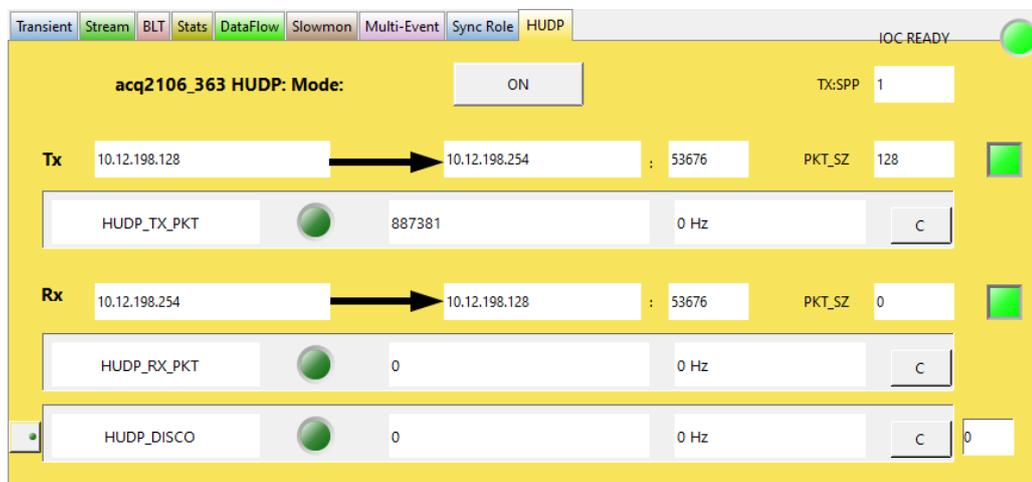
Figure 10: HUDP OPI showing TX packet count and RX variables set
