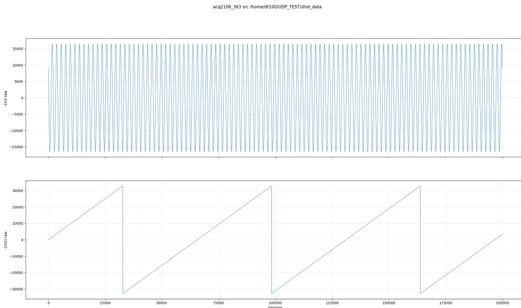
Figure 8: One whole seconds worth of data with zero packet loss
