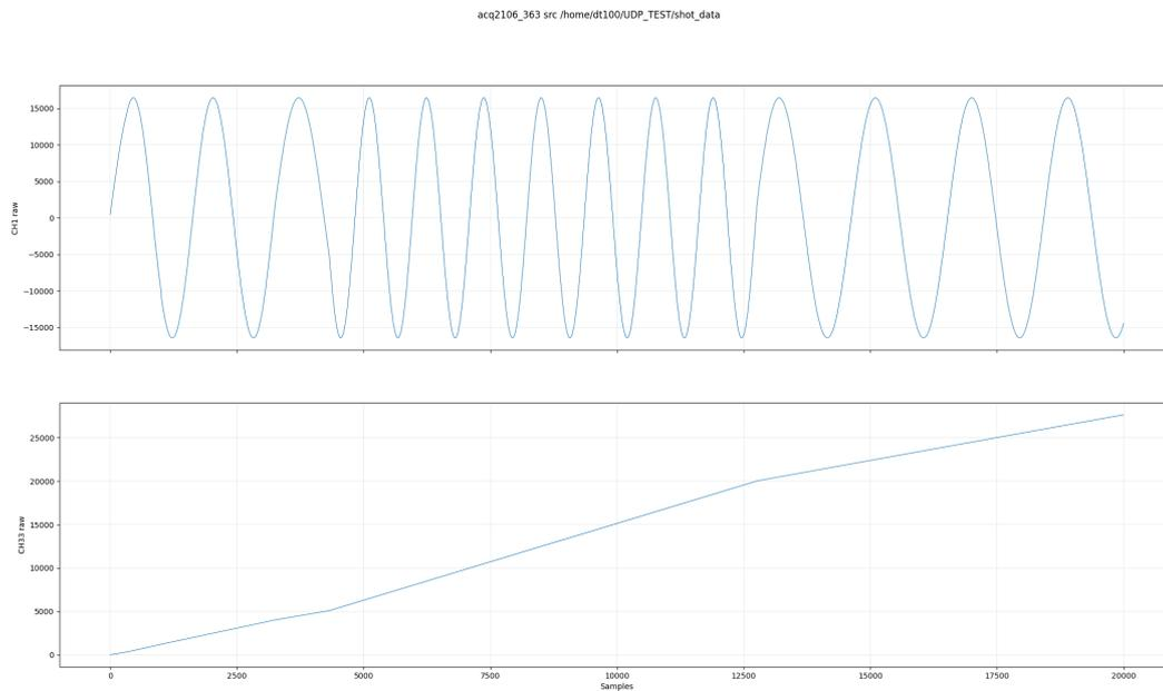
Figure 6: An example of packet loss when we overwhelm the host with too many packets per second
