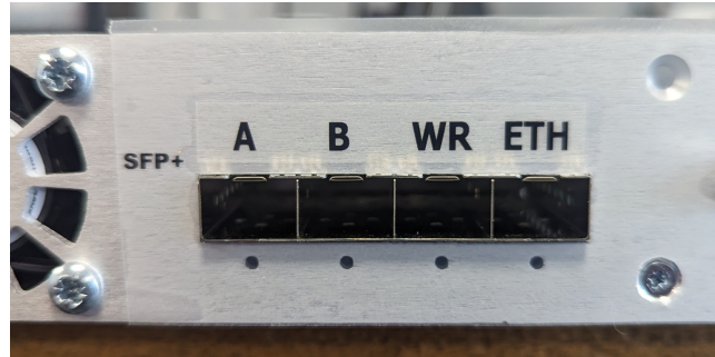
Figure 20: View of MGT482-SFP Ports
