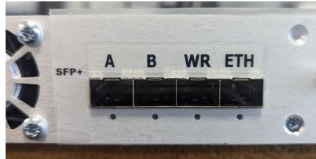
Figure 1: View of ACQ2106 MGT482-SFP Ports. Port D can be used for HUDP
