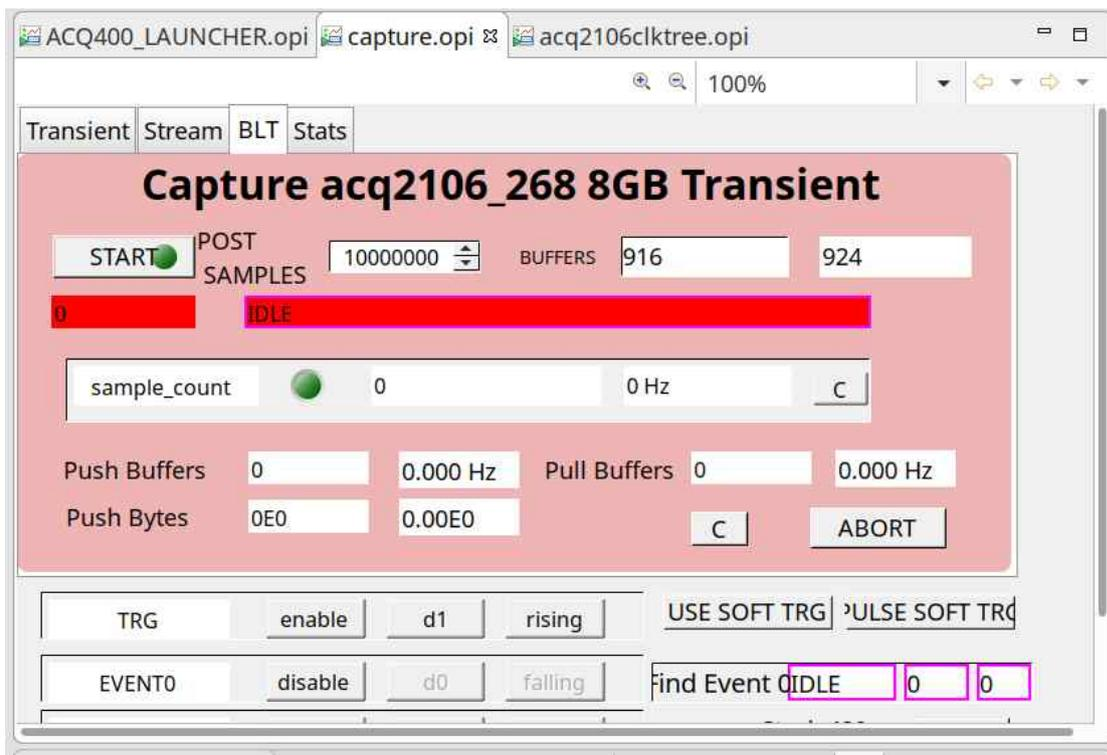
Showing POST=10,000,000, system calculation BUFFERS=916, rounded up to 924 buffers to allow offload to complete in groups of 12 (192 channel system).
