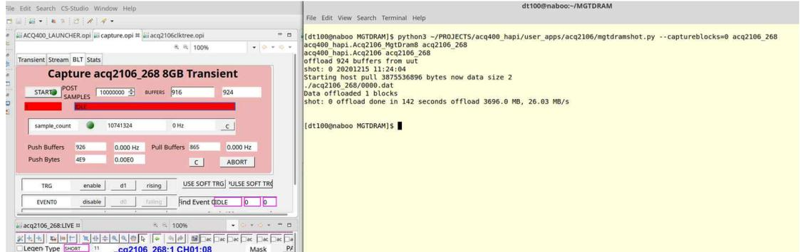
Data is stored to a numbered shotfile and rate displayed (26MB/s in this case).
