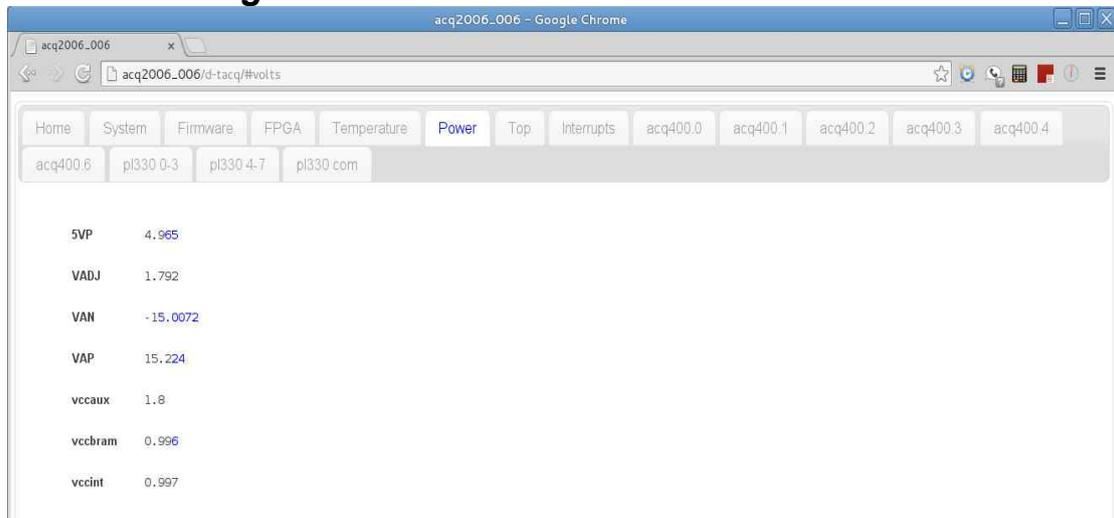
The screenshot shows a web browser window titled 'acq2006\_006 - Google Chrome'. The address bar shows 'acq2006\_006/d-tacq/#volts'. The navigation menu includes 'Home', 'System', 'Firmware', 'FPGA', 'Temperature', 'Power', 'Top', 'Interrupts', 'acq400.0', 'acq400.1', 'acq400.2', 'acq400.3', 'acq400.4', 'acq400.6', 'pl330 0-3', 'pl330 4-7', and 'pl330 com'. The 'Power' page displays the following data:
